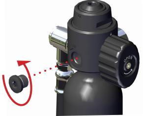
2. Remove the blanking plug from the 1st stage. Inspect the O-ring and attach the filling adapter to the 7/16" HP port where the blanking plug was mounted. Make sure the filling adapter is firmly attached. Attach the filling hose to the the filling adapter that corresponds to the max filling pressure stated on the cylinder neck.
