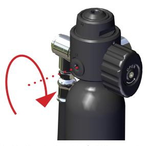
9. Mount the blanking plug in to the 7/16" HP port of the 1st stage and make sure it's firmly attached. Before mounting the blanking plug, inspect the o-ring to make sure it's without any flaws, make sure the o-ring is lubricated and that all sealing surfaces are clean and undamaged.
